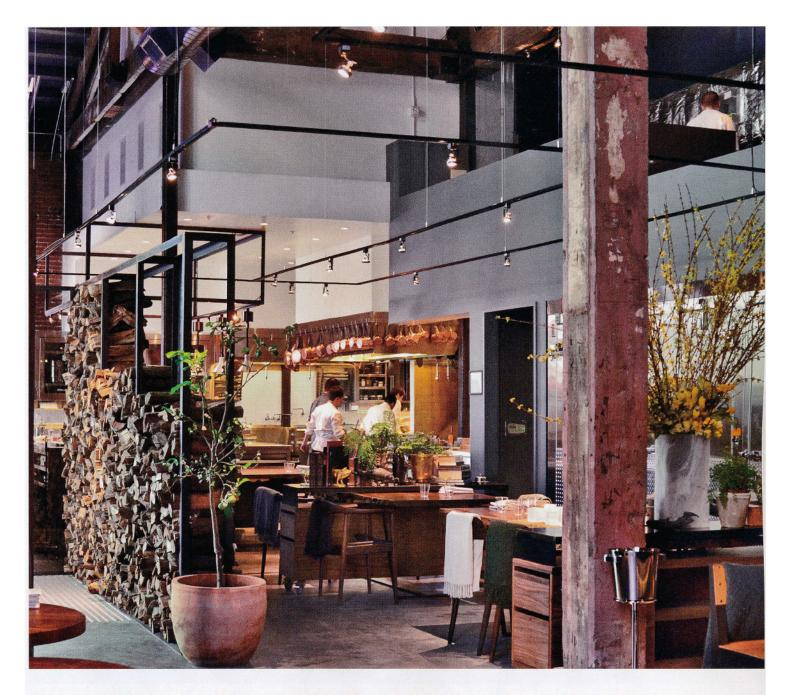
LED MR16 lamps. This system acts as a second ceiling by being physically lower, and creates a contrast between bright light and shadow to keep visitors' attention on one plane, much as a theater's lighting rig does. As Saison's primary source of illumination, the LEDs make the structure above the tracks seem to dissolve into the background. A coat of charcoal paint on the ceiling aids the disappearing act.
